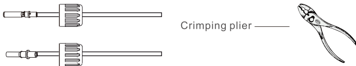
Pic 3.4 Crimp the contact pin to the wire
