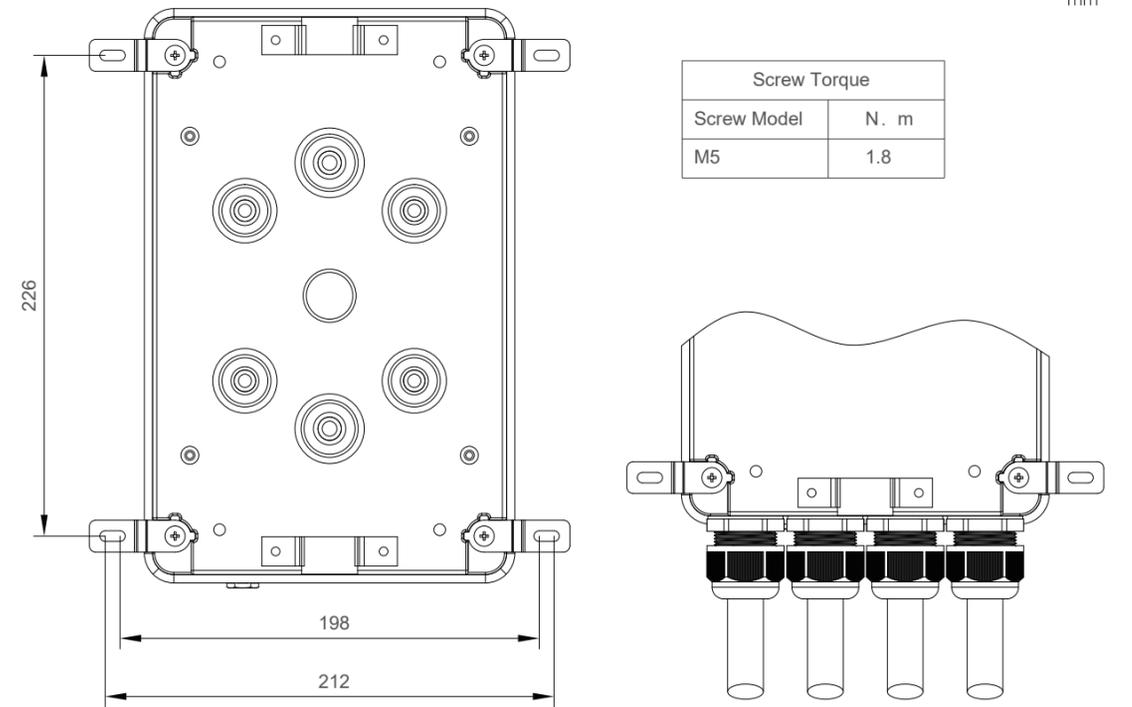
Fig 3 2-in 4-out mounting sizes drawings
