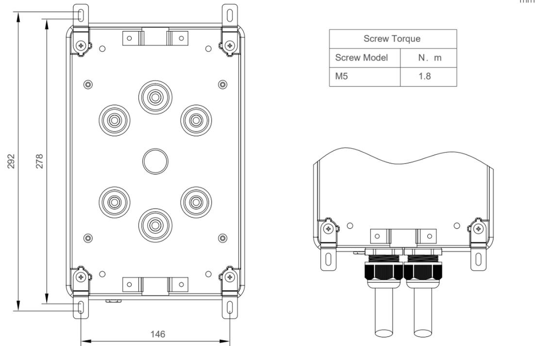
Fig 2 2-in 2-out mounting sizes drawings
