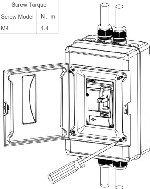
**Step 3** Fix the frame cover to the bottom base with M4 screw
