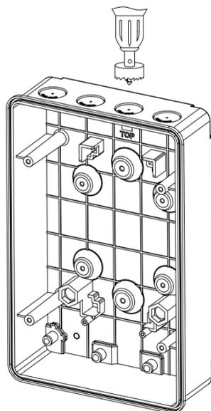
**Step 1** Open the hole on bottom with the hole opener according to the actual requirements, and install the cable gland after the hole opening is completed.
